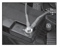
2. Unscrew the bolt of the red "+" battery terminal. Remove red tape from red "+" wires. Bolt the red wires to the red "+" terminal. Washers should be between the bolt and the wire. Red wires and terminal connection should appear as shown on left.
