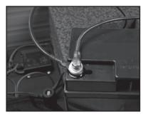
6. Unscrew the bolt from the "-" terminal and bolt in black "-" wires.
