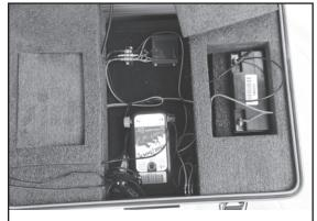
7. Place battery back into the foam pocket. The wires should be on top of the battery. Replace foam lid.
