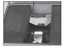
1. Looking at the inside of the PRS unit as in the picture, remove the left foam battery cover and set aside.
