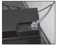
5. Remove right foam battery cover and set aside. Unscrew the bolt from the red "+" terminal of the battery. Remove red tape from red "+" wire and bolt to the terminal, use same method as step 2.
